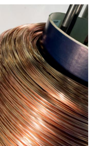
SIAT manufactures copper coated wires having diameters from 2 to 5 mm that can meet all market demands. Copper coated wires are cold rolled. Following reduction, wires undergo electrochemical pickling and then coppering so as to obtain fully adhering copper plating with variable thickness from 0.1 to 0.6 µm according to customers' requirements or specifications. All products are available in various packaging solutions up to a weight of 1000 kg.
